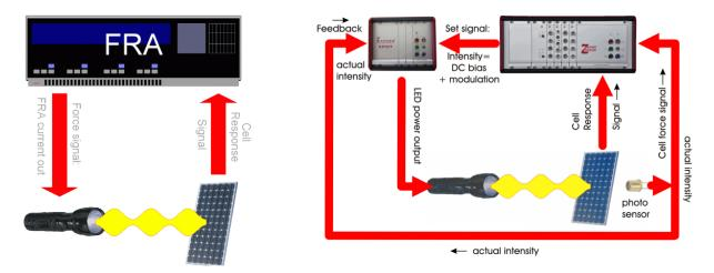
Fig. 4: Schematics of a tradition IMPS/IMVS setup and Zahner's CIMPS/CIMVS setup with feedback loop for controlled light illumination.
