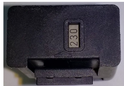
The selected main voltage is visible at the fuse holder bottom
