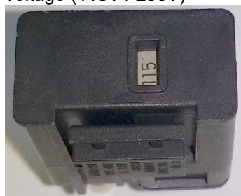
The selected main voltage is visible at the fuse holder bottom
