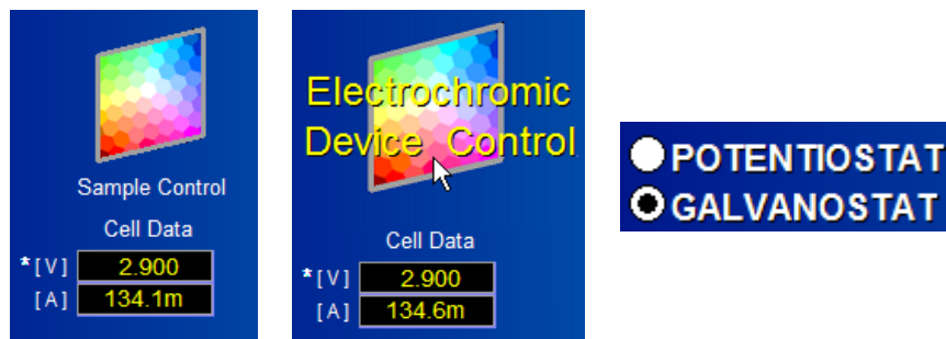
Fig. 23 Switching sample control to galvanostatic mode for charge scans
