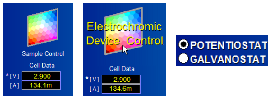
Fig. 20 Switching sample control to potentiostatic mode for voltage scans
