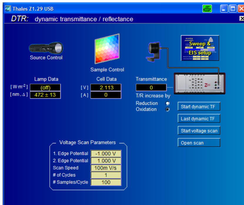
Fig. 3 Main window of CIMPS-dtr after startup
