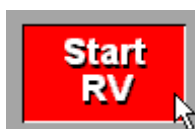
Fig. 15: A click on “Start RV” will trigger an RV measurement according to the conditions selected.
