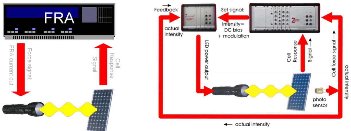
Fig. 4: Schematics of a tradition IMPS/IMVS setup and Zahner’s CIMPS/CIMVS setup with feedback loop for controlled light illumination.
