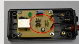
Randle circuit with NTC as Charge Transfer Resistance
