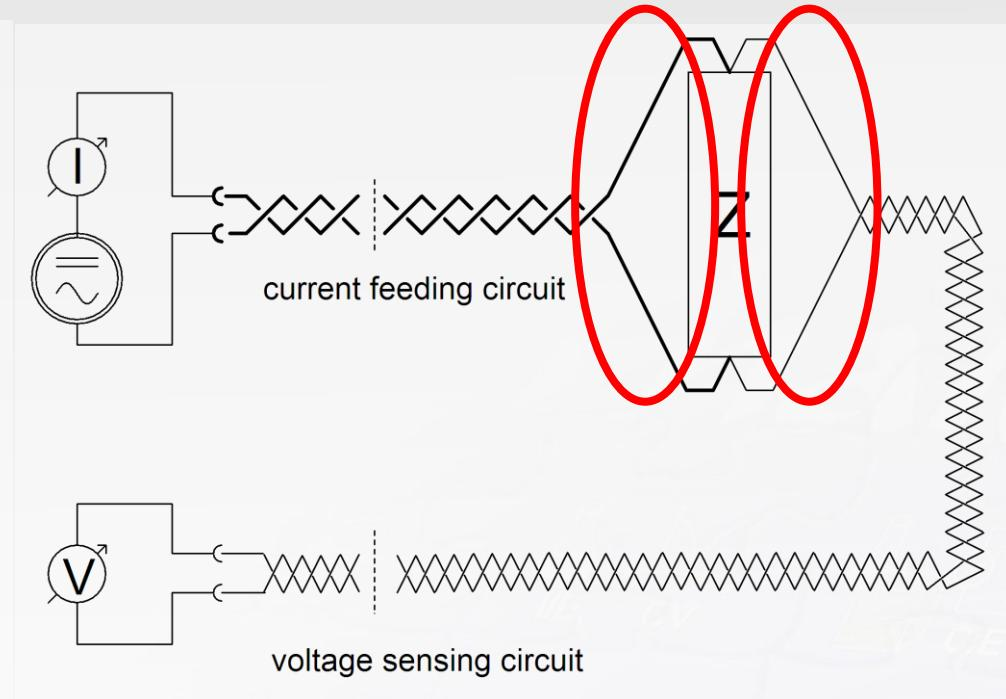
Interaction magnetical/electrical field => Drilling of Cables.
